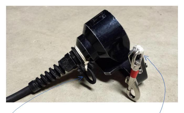
Bungee loop at back end of light/ballast for temp clip. Bungee loop is tied either with Fisherman's knot or just Overhead stopper knots at either end of bungee and in both cases, attached using "the knot"
