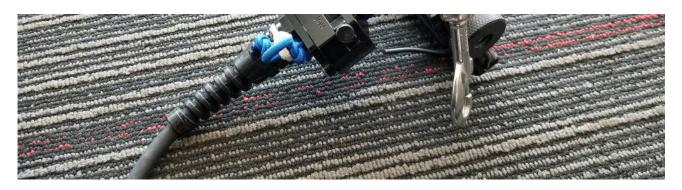
Below is a cordless light, here the light as a special tie off point allowing the bungee loop to be attached without having to secure it with "the knot."
