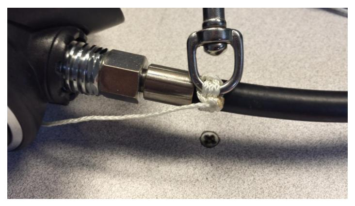
Step 6: Burn the tail of the cave line you just cut with the lighter until it forms a little ball of molten nylon. Using the back end of the lighter (or another tool, but NOT your fingers) smash the molten nylon into the knot, as pictured above.
